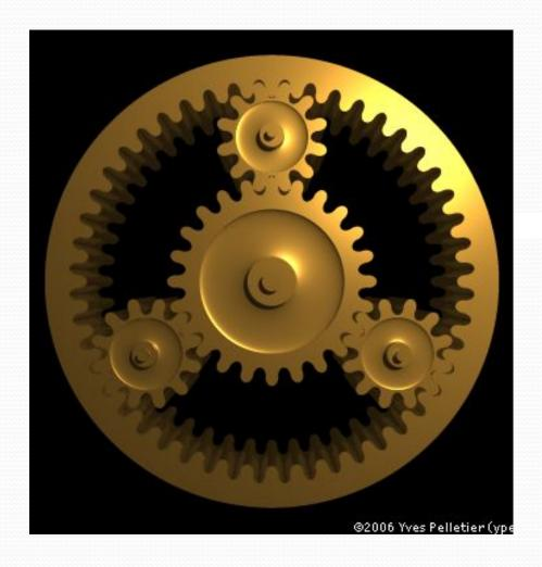
Planetary gear trains have several advantages. They have higher gear ratios. They are popular for automatic transmissions in automobiles. They are also used in bicycles for controlling power of pedaling automatically or manually. They are also used for power train between internal combustion engine and an electric motor.
